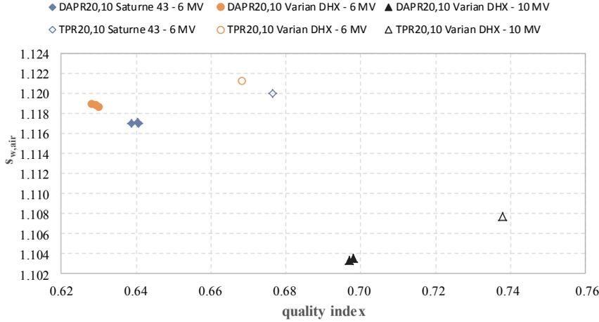
Fig. 6. Water-to-air stopping power ratio as a function of the beam quality index ( $DAPR_{20,10}^{R_{ref}}$  or  $TPR_{20,10}$ ). The stopping power ratios corresponding to  $DAPR_{20,10}^{R_{ref}}$  values (filled symbols) are calculated for the reference area ( $R = 1.5$  cm) while the stopping powers corresponding to  $TPR_{20,10}$  values (unfilled symbol) are calculated for a small volume on the beam axis.
