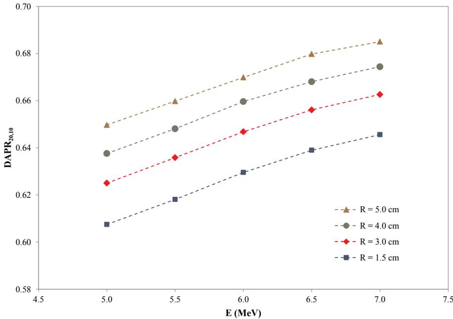
Fig. 3. Calculated  $DAPR_{20,10}$  with scoring region radii ( $R$ ) of 1.5 cm, 3 cm, 4 cm and 5 cm vs the initial electron beam energy used for the Monte Carlo simulation of the Varian 6 MV beam with diameter of 1.25 cm.
