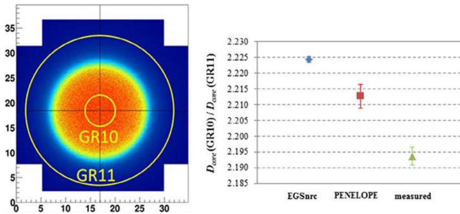
Fig. A1. Left hand side, representation of the core diameters for the GR11 and GR10 calorimeters (yellow circles) in a 2 cm diameter beam (measured with EBT3 films) and right hand side,  $D_{core}(GR10)/D_{core}(GR11)$  ratios measured and calculated with EGSnrc and PENELOPE (error bars are type A uncertainties at one standard deviation).
