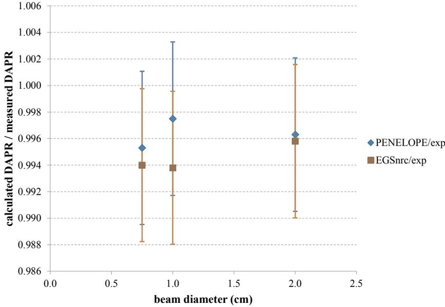
Fig. 5. Ratios of calculated  $DAPR_{20,10}$  to measured  $M(20)/M(10)$  for a scoring region corresponding to a disc of 3 cm diameter. The uncertainties correspond to one standard deviation including the statistical and estimated (0.55%) uncertainties.
