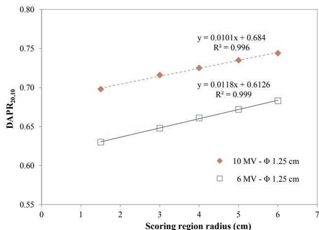
**Fig. 2.** Monte Carlo calculated  $DAPR_{20,10}$  with SDD 100 cm as a function of the scoring region radius,  $R$ , for the 6 MV and 10 MV stereotactic beams with diameter 1.25 cm produced by the Varian DHX accelerator.
