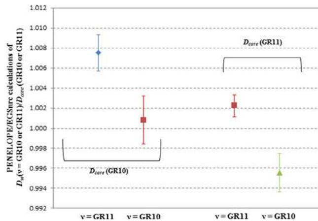
Fig. A2.  $(D_w(v)/D_{core})_{PENELOPE} / (D_w(v)/D_{core})_{EGSnrc}$  for cores and volumes of water  $v$  corresponding to the GR10 and GR11 calorimeter cores (error bars are type A uncertainties at one standard deviation).
