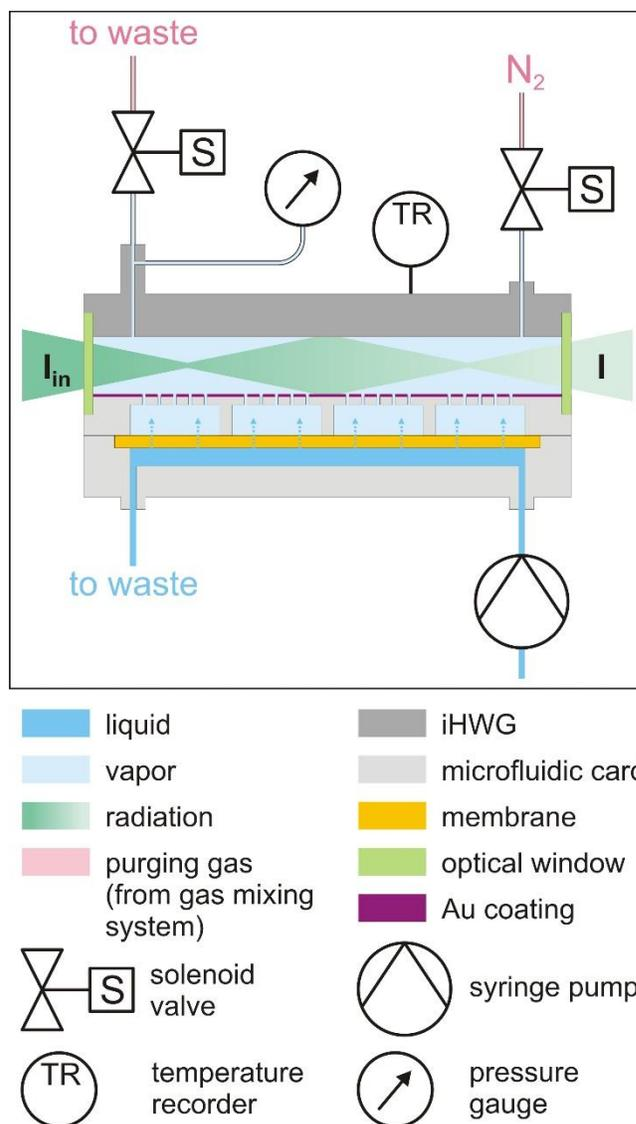
Fig. 1. Schematic cross-section of the experimental setup (not to scale).  $I_{in}$ : intensity of the in-coupled radiation (emanating from the FTIR spectrometer). Snapshot during the acquisition of a single-channel sample spectrum (i.e., both solenoid valves closed; equilibration phase).  $I$ : out-coupled radiation intensity;  $I < I_{in}$  due to the presence of absorbing molecules within the IR beam path within the iHWG.
