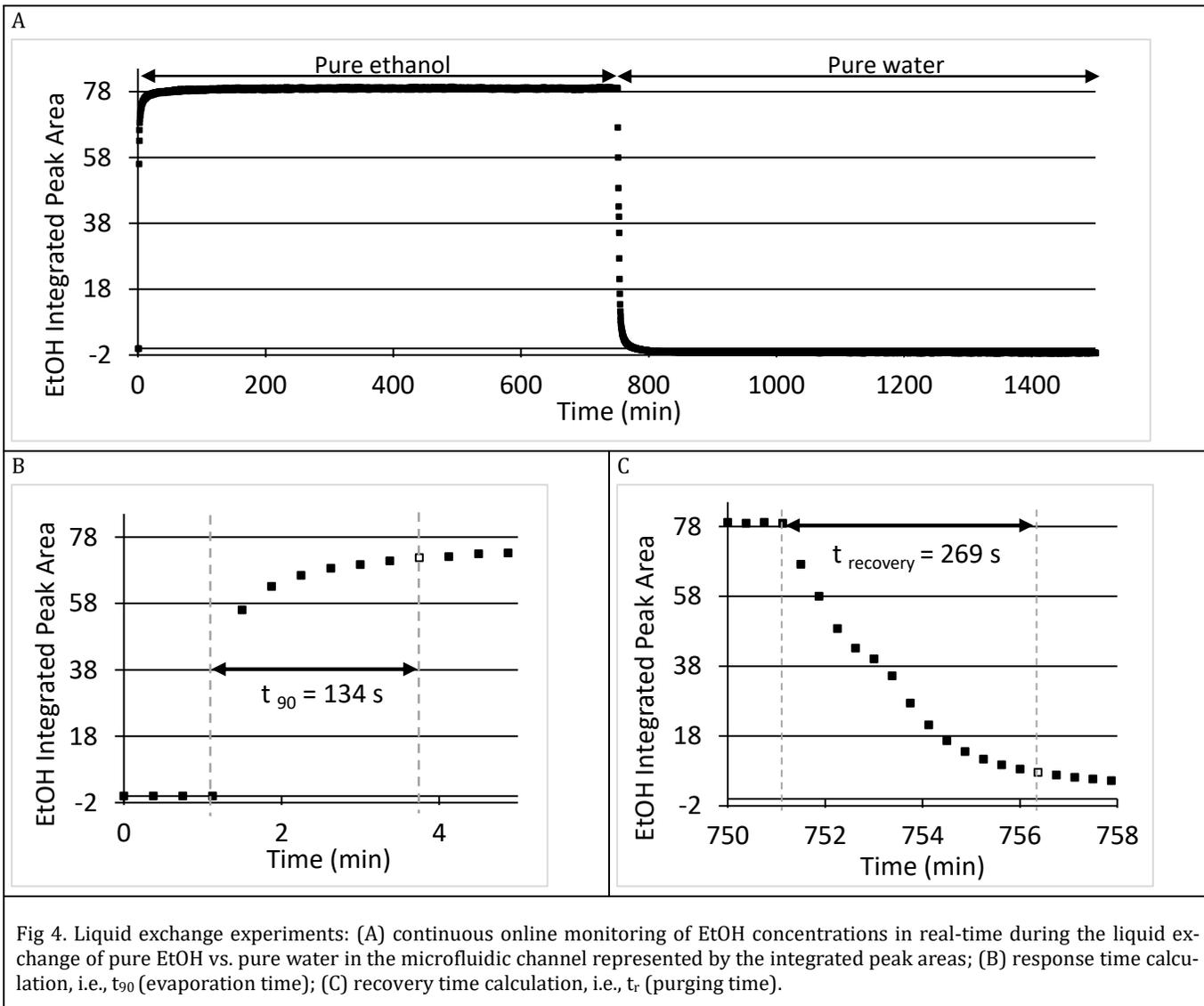
Fig 4. Liquid exchange experiments: (A) continuous online monitoring of EtOH concentrations in real-time during the liquid exchange of pure EtOH vs. pure water in the microfluidic channel represented by the integrated peak areas; (B) response time calculation, i.e.,  $t_{90}$  (evaporation time); (C) recovery time calculation, i.e.,  $t_r$  (purging time).
