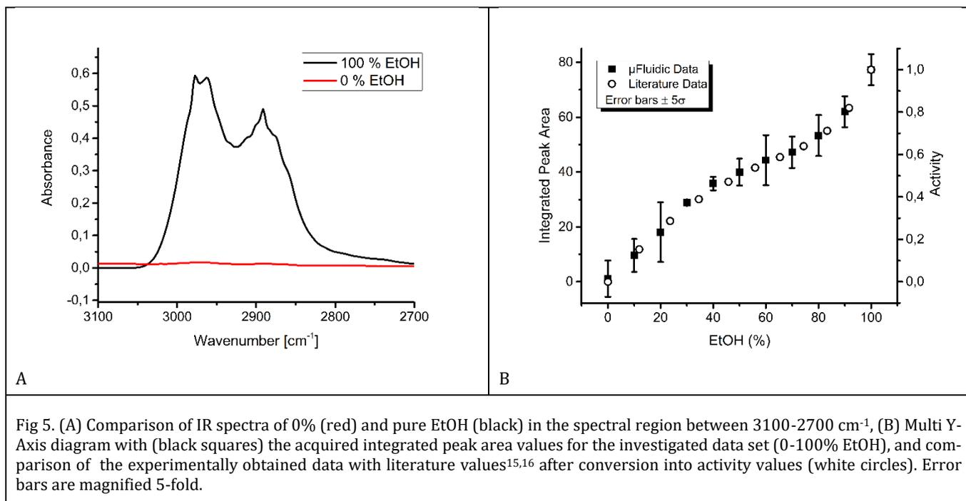
Fig 5. (A) Comparison of IR spectra of 0% (red) and pure EtOH (black) in the spectral region between 3100-2700  $\text{cm}^{-1}$ , (B) Multi Y-Axis diagram with (black squares) the acquired integrated peak area values for the investigated data set (0-100% EtOH), and comparison of the experimentally obtained data with literature values<sup>15,16</sup> after conversion into activity values (white circles). Error bars are magnified 5-fold.
