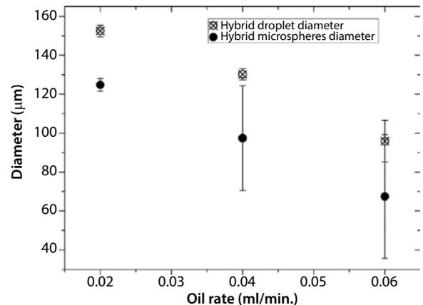
**Figure 4** Size of hybrid chitosan-collagen emulsion droplets (crossed open circle) and microspheres after ammonia vapors (solid circles) as a function of oil flow rate at constant chitosan solution flow rate ( $0.002 \text{ ml}\cdot\text{min}^{-1}$ ). Chip  $100 \times 100 \mu\text{m}^2$  cross design.
