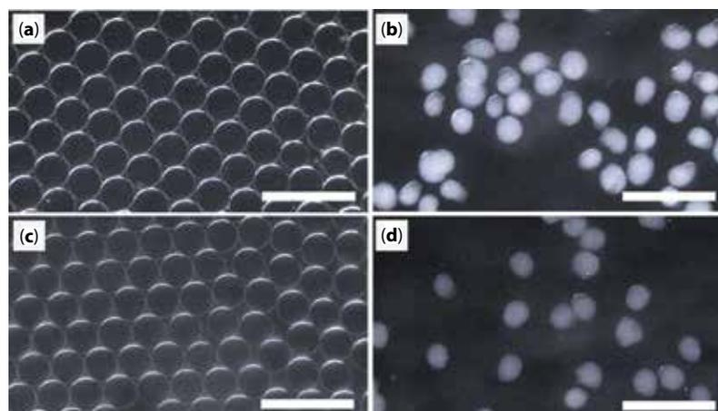
**Figure 2** Images of emulsion droplets and microspheres generated with the T-junction millifluidic device: (a) chitosan emulsion, (b) chitosan microspheres after ammonia vapors, (c) chitosan-collagen hybrid emulsion, (d) hybrid microspheres after ammonia vapors. Micrographs (a–d) were taken under darkfield illumination. Scale bar: 500  $\mu\text{m}$ .
