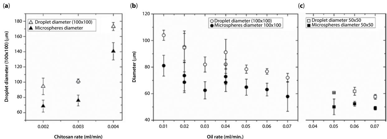
**Figure 3** Size of emulsion droplets (open symbols) and microspheres after ammonia vapors (solid symbols): (a) as a function of chitosan solution flow rate at constant oil flow rate ( $0.02 \text{ ml}\cdot\text{min}^{-1}$ ) and (b) as a function of oil flow rate at constant chitosan solution flow rate ( $0.002 \text{ ml}\cdot\text{min}^{-1}$ ). The emulsion was obtained on a microfluidic chip with a  $100 \times 100 \mu\text{m}^2$  (a, b) or  $50 \times 50 \mu\text{m}^2$  (c) cross design.
