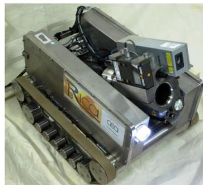
**Figure 5:** Example of a module grouping instruments for the location and radiological characterization of hot spots (DUCROS, HAUSER, Majhoubi, & GIRONES, 2016)
