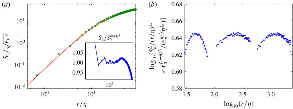
FIGURE 3. (Colour online) (a) Non-dimensionalized second-order structure function ( $S_2/(\epsilon_v \nu)^{1/2}$ ) from case A. Comparison with the Sirovich model. Inset: discrepancy between the two curves (ratio of  $S_2$  to the model). Close agreement between the two implies an accurate estimate of  $\epsilon_v$  (for case A). The experimental noise in  $S_2$  is partially removed by subtracting a value of 0.2. (b) Third-order structure function compensated by power 1.
