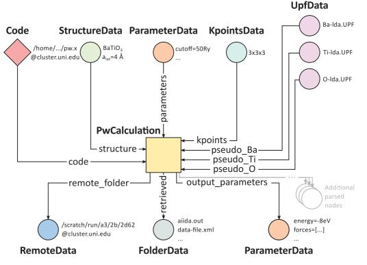
Figure 4. A simple AiiDA directed acyclic graph for a QUANTUM ESPRESSO calculation using PWscf (square), with all the input nodes (data, circles; code executable, diamond) and all the output nodes that the daemon creates and connects automatically.
