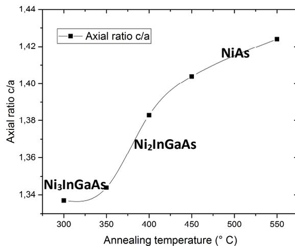
Figure 4. Evolution of the c/a lattice parameters ratio of the intermetallic according to temperature
