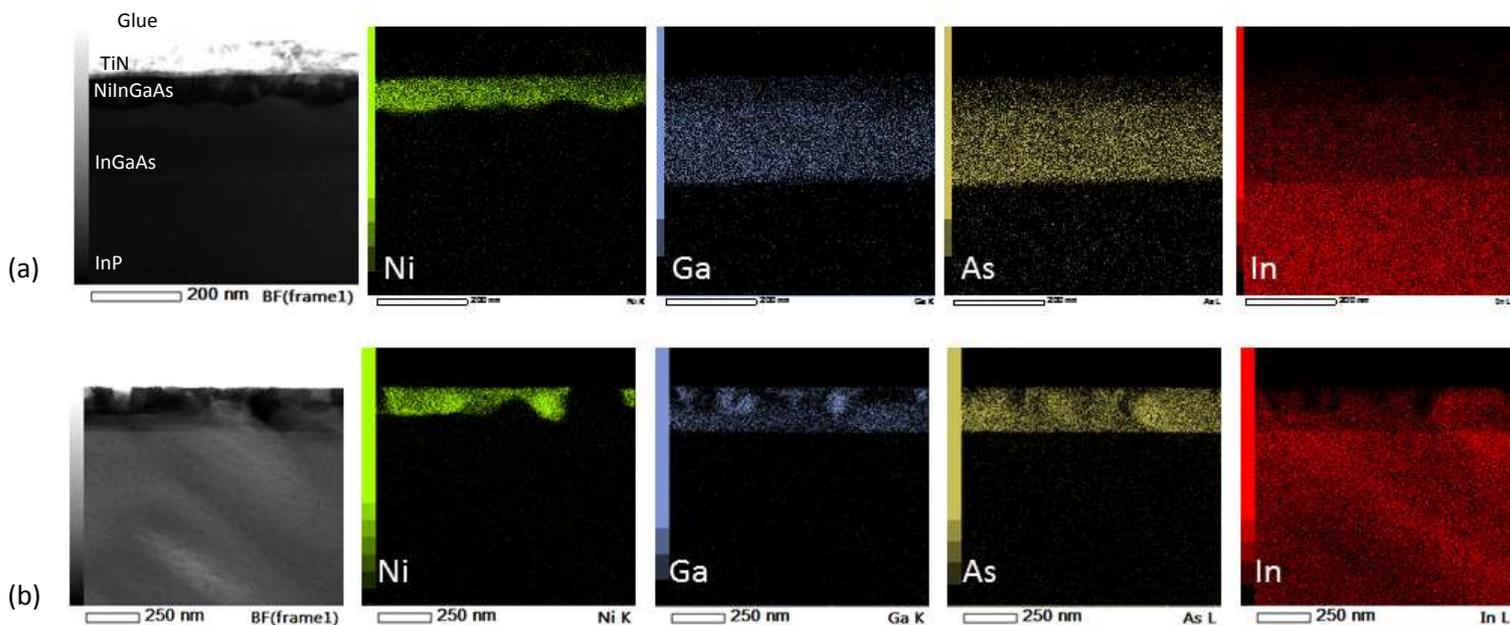
Figure 5 : (a) TEM and EDX images of the sample annealed at 300 °C (b) TEM and EDX images of the sample annealed at 550 °C
