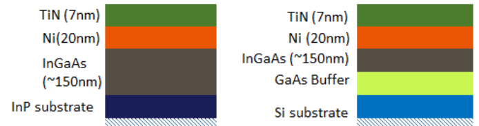
Fig. 1. Scheme of the as-deposited stacks of the prepared samples: (a) TiN/Ni/InGaAs/InP, (b) TiN/Ni/InGaAs/GaAs/Si.
