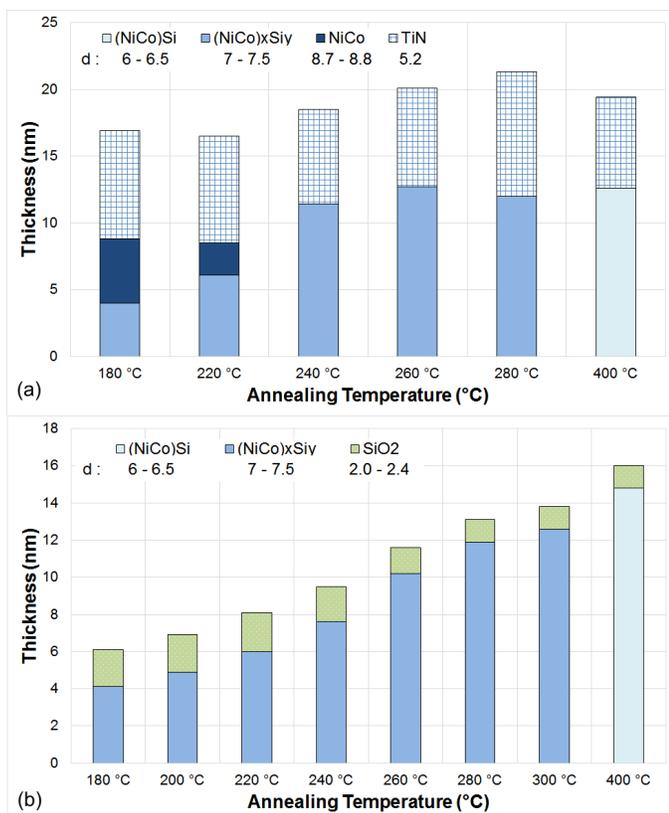
Fig. 2. XRR spectra modelling without selective etching (a) and with selective etching (b) of  $\text{TiN}$  (7 nm) /  $\text{Ni}_{0.9}\text{Co}_{0.1}$  (7 nm) / Si samples at various annealing temperatures.
