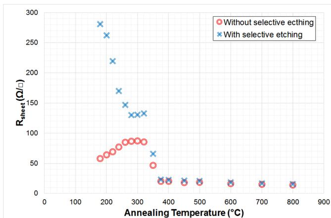
Fig. 1. Sheet resistance measured after annealing  $\text{Ni}_{0.9}\text{Co}_{0.1}$  (7 nm) on Si substrate at various temperatures for 30 s under  $\text{N}_2$ . The sheet resistances of annealed samples with and without selective etching are indicated by crosses and circles, respectively.
