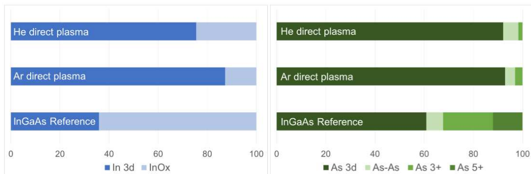
Figure 2. Relative spectral weight of the components determined for InGaAs samples with various surface treatments for In 3d (left) and As 3d (right) regions.
