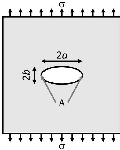
**Figure 1.** Sketch of Inglis's plate under stress ( $\sigma$ ) with an elliptical hole in it (recreated from [41]; for more details see [41–43]). The parameters  $a$  and  $b$  represent the length of the semi-major and semi-minor axis of the hole. Stresses concentrate at the vertices of the semi-major axis (i.e. points A in the figure). The radius of curvature at A is  $\rho_A$ .
