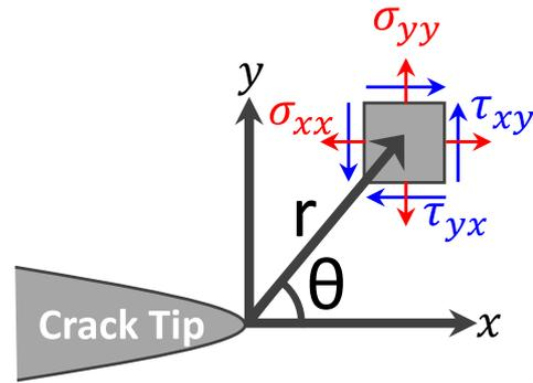
**Figure 2.** Sketch of the stress field around a crack tip in polar coordinates— $r$  is the distance from the crack tip and  $\theta$  is the polar angle. The variables  $\sigma_{ij}$  and  $\tau_{ij}$  represent the normal and shear components of the stress, respectively. Reproduced with permission from [10, 43].
