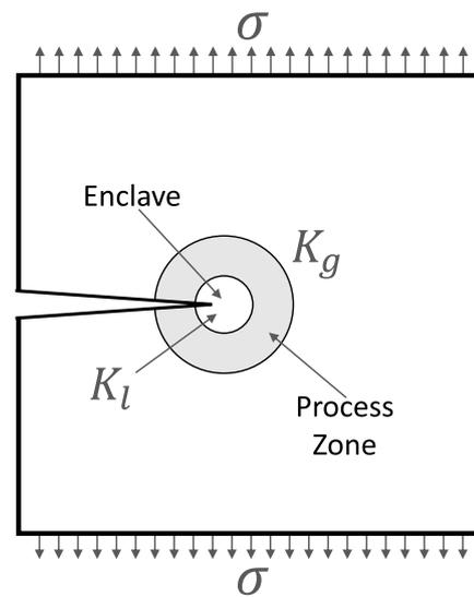
**Figure 5.** Sketch of the  $K$ -field felt by the crack tip (recreated from [41]).  $K_I$  represents the stress intensity factor in the local region around the crack tip, or the enclave.  $K_g$  represents the global (or continuum) stress intensity factor.
