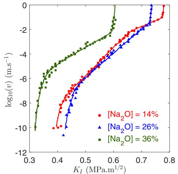
**Figure 19.** Semi-log plot of the crack front velocity,  $v$ , as a function of the stress intensity factor,  $K_I$ . These results correspond to Gehrke *et al* 1991 study of stress corrosion cracking in [SiO<sub>2</sub>–[Na<sub>2</sub>O]–[Al<sub>2</sub>O<sub>3</sub>]] (SNA) glasses in a liquid water environment. [54] © Chapman and Hall 1991. With permission of Springer.
