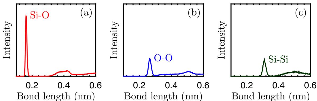
**Figure 8.** Pair distribution function as a function of bond length. Figures in panels correspond to the distribution of: (a) Si–O bond length, (b) O–O bond length, and (c) Si–Si bond length. Bond lengths are based on molecular dynamics simulations of pure-amorphous silica with  $\sim 5000$  atoms in the system (for simulation details see [43, 78–81]). Simulations invoke the Vashishta *et al* potential [82, 83].
