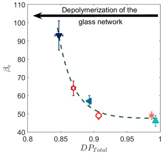
**Figure 27.** Slope in Region I ( $\beta_c$ ) as a function of the total degree of polymerization ( $DP_{Total}$ ) of the glass network. Reprinted from [65], with permission from Elsevier.  $DP_{Total} = 1$  represents a full polymerized system.  $DP_{Total} < 1$  represents a system with some degree of depolymerization.
