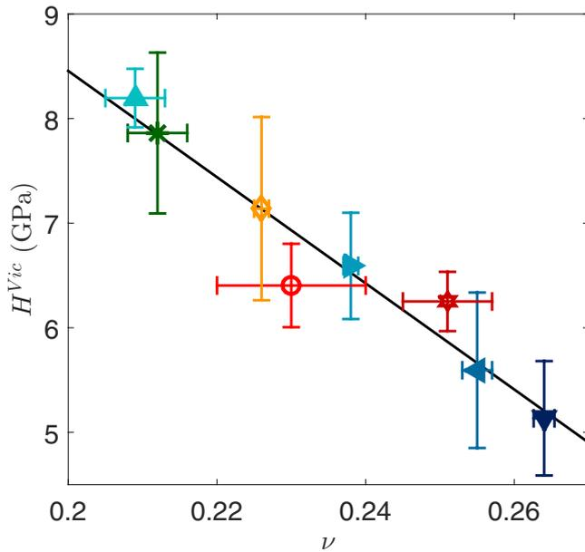
**Figure 16.** Hardness,  $H^{Vic}$ , of SBN glasses as a function of their Poisson's ratio,  $\nu$ . Table 11 provides the chemical composition of each point. Each point arises from an average over maximum loads of 50 and 100g. The line indicates a linear fit of the data:  $H^{Vic} = -51_{\pm 5} \times \nu + 19_{\pm 1.3}$ .
