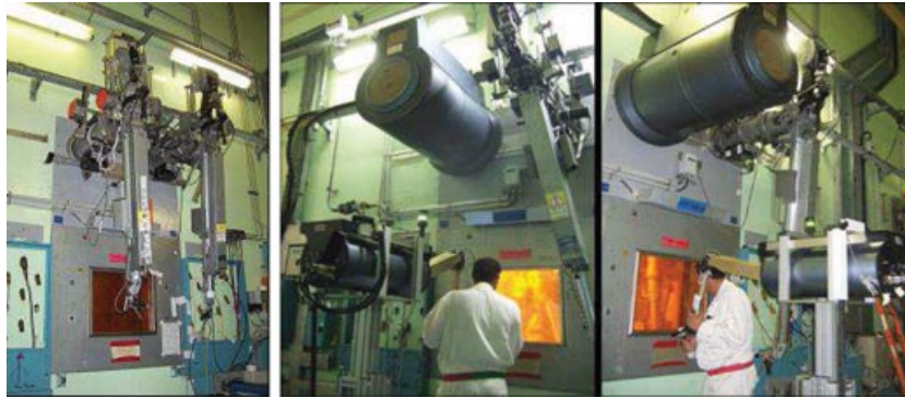
Figure 19. Virtuose 6D 40-40 [a conventional workstation (left)], and a mixed workstation equipped with the new MT200 TAO telerobot and a standard MT200 MSM (right).
