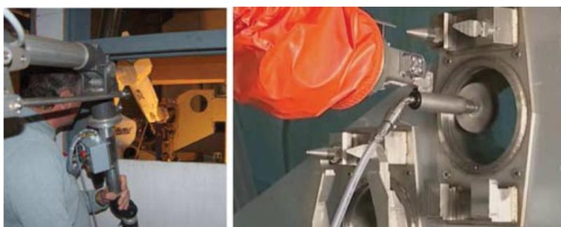
Figure 16. Brushing task on the mock-up.
