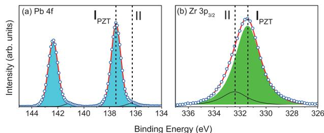
FIG. 3. (a) Pb 4f and (b) Zr 3p<sub>3/2</sub> spectra. The Pb components are in cyan and the Zr components are in green. The label I represents Pb/Zr in PZT, whereas label II identifies reduced Pb or Zr in surface nanostructures, respectively.
