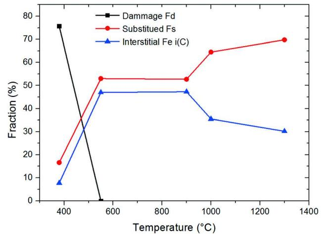
FIG. 3. Evolution of the Fe atoms fractions in the substitutional and interstitial sites versus temperature.
