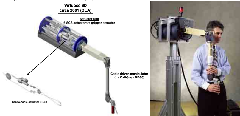
Fig 3. Left, Virtuose 6D the first 6 axis force feedback master arm powered by screws and cables – Right, V6D 4040 an industrial version produced Haption®
