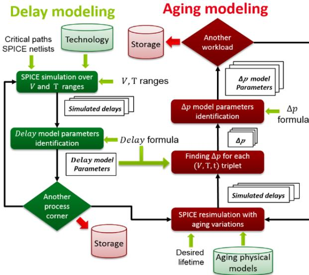
Figure 1. Methodology for obtaining a circuit-level aging model from device-level models. The first step consists in generating a propagation delay model  $Delay(V, T)$ . Aging simulations are then conducted to find the parameter shift  $\Delta p$ . A  $\Delta p(V, T, t)$  formula is constructed at the end. All parameters from both  $Delay$  and  $\Delta p$  formula are stored to be used during circuit operation.
