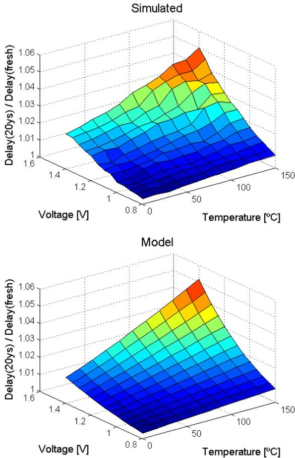
Figure 7. Degradation surfaces constructed through SPICE simulations (top) and the proposed models (bottom) for a power-on time of 20 years. The  $V, T$  conditions are the same for both delay and aging, this is why there is almost no degradation at low  $V$  and  $T$ .
