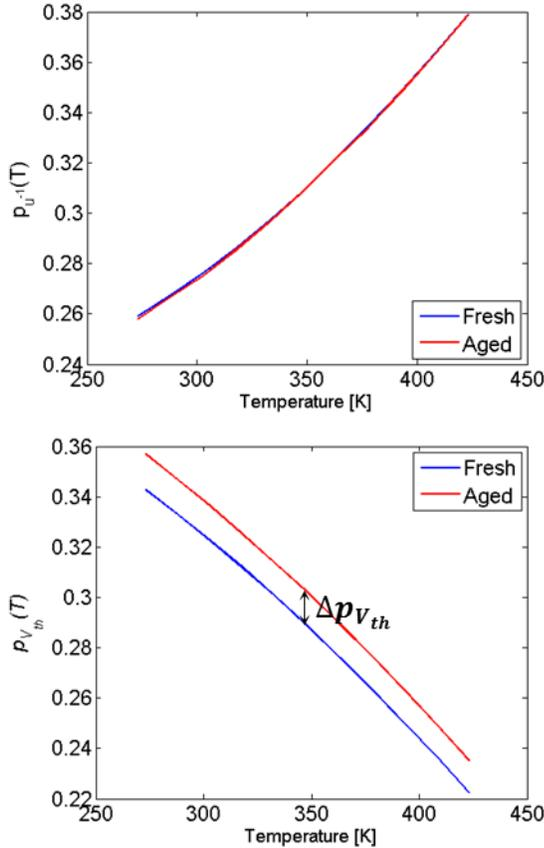
Figure 4. Evolution of  $p_{\mu^{-1}}(T)$  and  $p_{V_{th}}(T)$  from a fresh situation to an aged one (10 ys, 150°C, 1.2V). There is no significant change of  $p_{\mu^{-1}}$ , while  $p_{V_{th}}$  shows a shift due to aging ( $\Delta p_{V_{th}}$ ).
