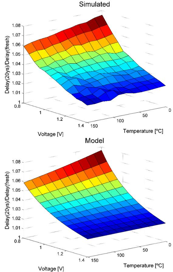
Figure 8. Similar to Figure 7, degradation surfaces constructed through SPICE simulations (top) and the proposed models (bottom) but with a fixed  $\Delta p_{V_{th}}$  corresponding to a stress condition of 1.2V, 125°C and 20 years.
