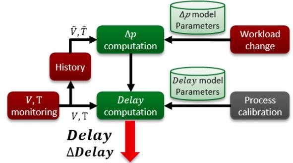
Figure 2. On-line estimation of circuit degradation from previously created models. Process calibration is done only once at the beginning of circuit lifetime.  $V, T$  and workload are constantly monitored to keep  $\Delta p$  up-to-date. Both  $Delay$  and  $\Delta Delay$  are calculated upon request, the last being the delay shift induced by BTI/HCI effects ( $\Delta p$ ).
