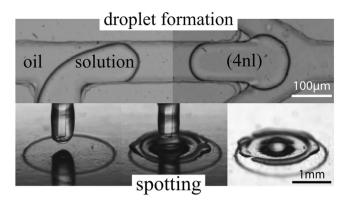
**Figure 1.** DMF-MALDI Set-up: droplet creation and spotting. Top: droplet generation (left), droplet spacing (right) within the PDMS microfluidic chip. Bottom: before deposition (left), during deposition (middle), after deposition (right) on stainless steel MALDI plate.
