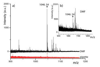
**Figure 4.** MALDI-TOF MS spectra of: (**a**) a 0.5 nM solution of Ang II spotted by DMF (black line) and standard pipette (red line shifted for clarity), and (**b**) DMF spotting of 0.1 nM solution of Ang II.
