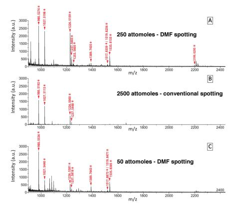
**Figure 5.** MALDI-TOF MS spectra of MMP12 digest: (**A**) DMF deposition of 250 attomoles, (**B**) Conventional pipette deposition of 2500 attomoles, (**C**) DMF deposition of 50 attomoles. The ticked masses and star-labeled peaks correspond to tryptic fragments of MMP12.
