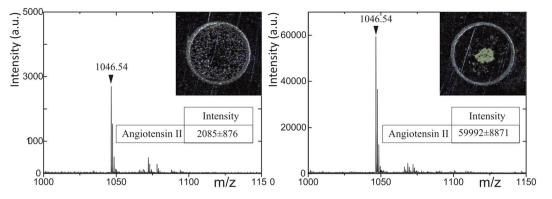
**Figure 2.** MALDI-TOF MS spectra of 5 femtomoles of Ang II. Left. Standard pipette deposition. Right. DMF deposition. Inserts: Dried mixture of peptide/matrix before laser desorption.
