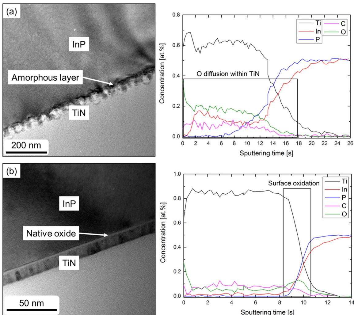
FIG. 7. Bright field TEM images and corresponding AES depth profiles of TiN (7 nm)/InP samples (a) after an HCl:  $\text{H}_2\text{O} = 1: 2$  wet surface preparation combined with an *in situ*  $\text{Ar}^+$  plasma treatment and (b) after an HCl:  $\text{H}_2\text{O} = 1: 2$  wet surface preparation.
