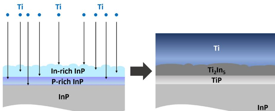
FIG. 8. Schematic representation of the formation of the Ti<sub>2</sub>In<sub>5</sub> and TiP phase during the deposition process.
