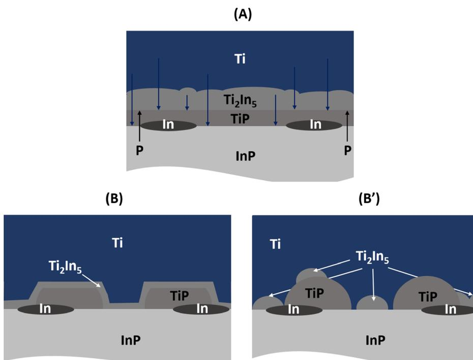
FIG. 10. Schematic representation of the three situations that could enable the species to interact during the annealing treatment conducted at 550 °C with (A) the diffusion of the species through the TiP and  $\text{Ti}_2\text{In}_5$  layers, (B) the agglomeration of the TiP layer and (B') the agglomeration of the TiP and  $\text{Ti}_2\text{In}_5$  layers. Note that these diagrams represent the intermediate states occurring throughout the annealing process.
