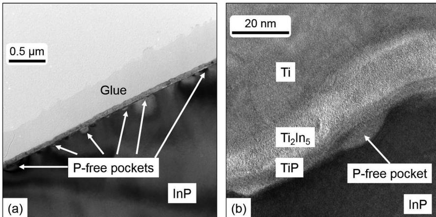
FIG. 9. TEM cross section of the as deposited TiN (7 nm)/Ti (20 nm)/InP system showing the presence of P-free pockets below the TiP layer.
