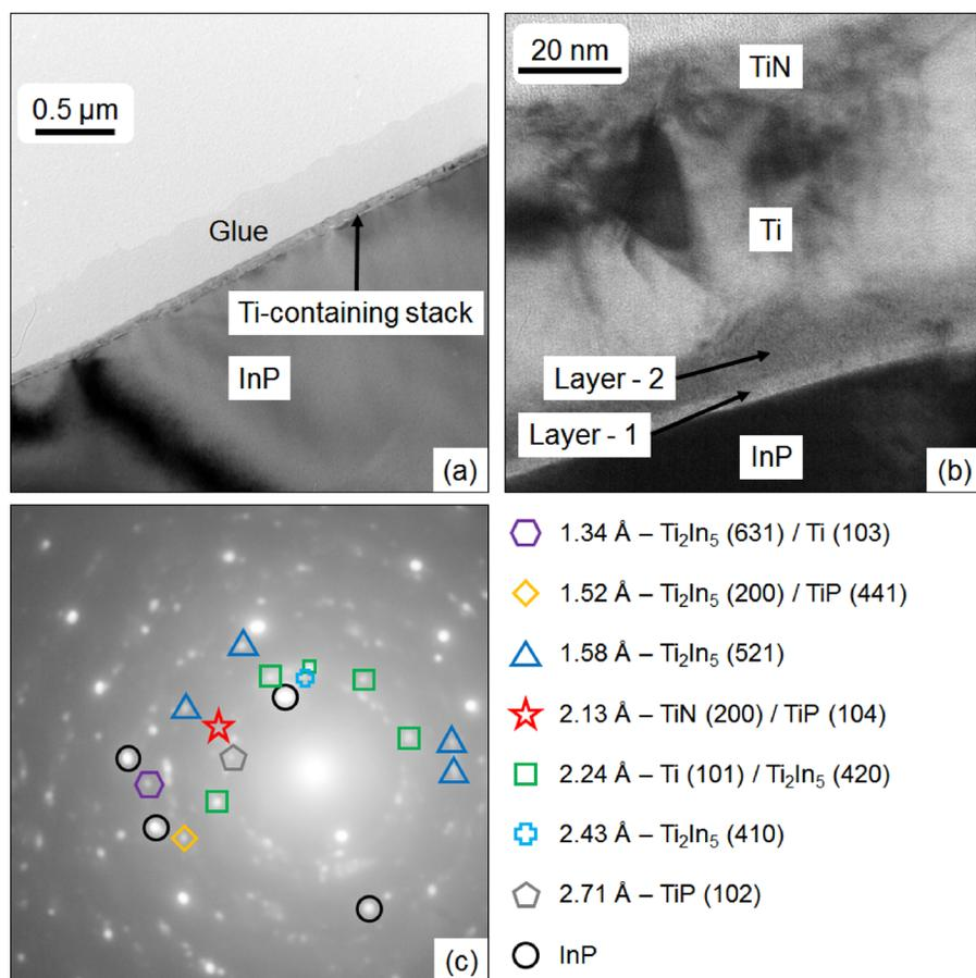
FIG. 2. Bright field TEM cross section of (a) the TiN (7 nm)/Ti (20 nm)/InP as deposited sample in low magnification, (b) the TiN (7 nm)/Ti (50 nm)/InP as deposited sample in high magnification and (c) the corresponding SAED pattern highlighting the presence of four different layers in the system.
