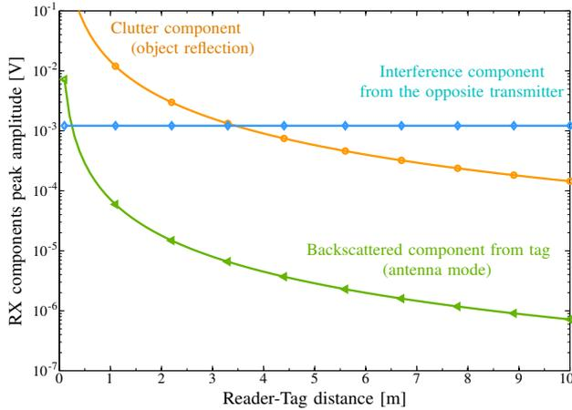
Fig. 6. Typical dynamic range of a UWB-RFID system.
