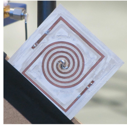
Fig. 6. Single port UHF/UWB antenna prototype on paper substrate [28].
