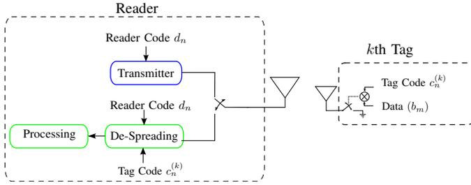
Fig. 2. Reader-Tag considered architectures for detection and communication.
