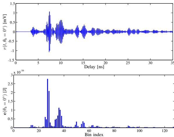
Fig. 5. Accumulated received signal using the receiver A and energy profile using the receiver B over  $N_p = 100$  pulses.
