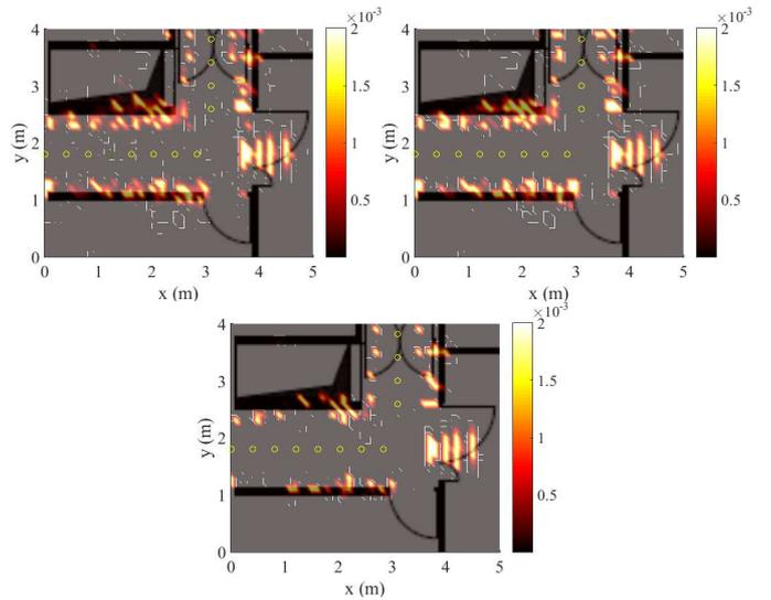
Fig. 8. Cleaning approach for  $W = 3 \text{ GHz}$ . RCS results for  $N_p = 100$ , cell size  $0.1 \times 0.1 \text{ m}^2$ ,  $MR = 15 \text{ m}$ . Top-left: Approach 1. Top-right: approach 2. Bottom: approach 3.
