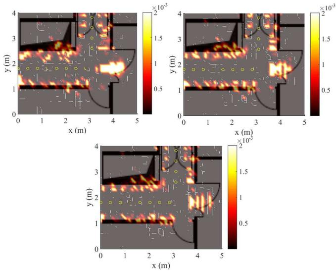
Fig. 3.  $W$  impact. RCS results for  $N_p = 100$ , cell size  $0.1 \times 0.1 \text{ m}^2$ ,  $MR = 15 \text{ m}$  and no cleaning. Top-left:  $W = 1 \text{ GHz}$ . Top-right:  $W = 2 \text{ GHz}$ . Bottom:  $W = 3 \text{ GHz}$ .
