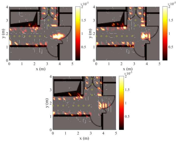
Fig. 5.  $N_p$  impact. RCS results for  $N_p = 30$ , cell size  $0.1 \times 0.1 \text{ m}^2$ ,  $MR = 15 \text{ m}$  and no cleaning. Top-left:  $W = 1 \text{ GHz}$ . Top-right:  $W = 2 \text{ GHz}$ . Bottom:  $W = 3 \text{ GHz}$ .
