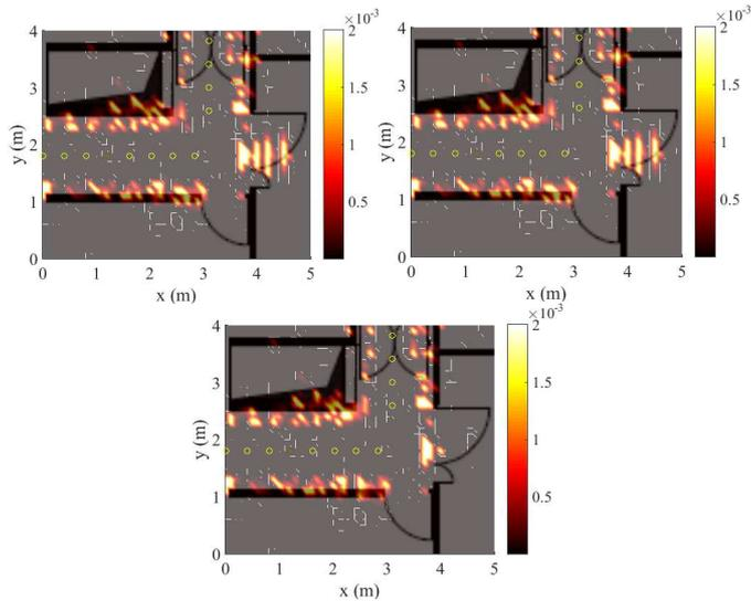
Fig. 6. Maximum range impact for  $W = 3 \text{ GHz}$ . RCS results for grid cell size  $0.1 \times 0.1 \text{ m}^2$  and  $N_p = 100$ . Top-left:  $MR = 10 \text{ m}$ . Top-right:  $MR = 5 \text{ m}$ . Bottom:  $MR = 2 \text{ m}$ .
