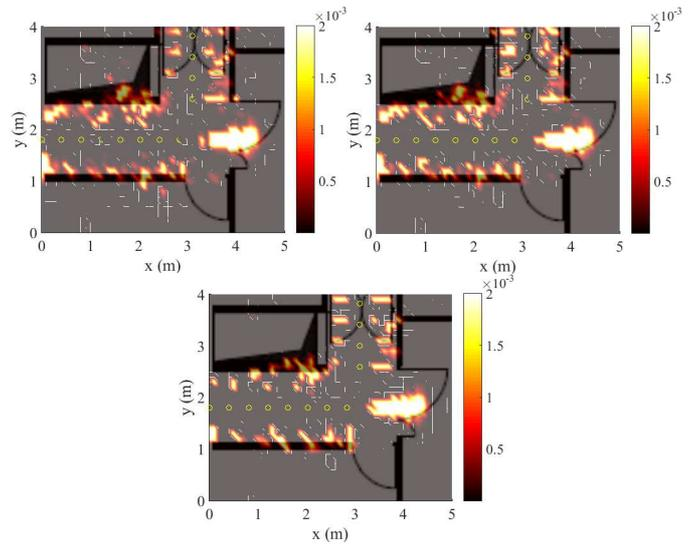
Fig. 7. Cleaning approach for  $W = 1 \text{ GHz}$ . RCS results for  $N_p = 100$ , cell size  $0.1 \times 0.1 \text{ m}^2$ ,  $MR = 15 \text{ m}$ . Top-left: approach 1. Top-right: approach 2. Bottom: approach 3.
