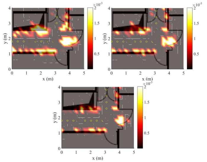
Fig. 4. Cell size impact. RCS results for  $N_p = 100$ , cell size  $0.2 \times 0.2 \text{ m}^2$ ,  $MR = 15 \text{ m}$  and no cleaning. Top-left:  $W = 1 \text{ GHz}$ . Top-right:  $W = 2 \text{ GHz}$ . Bottom:  $W = 3 \text{ GHz}$ .
