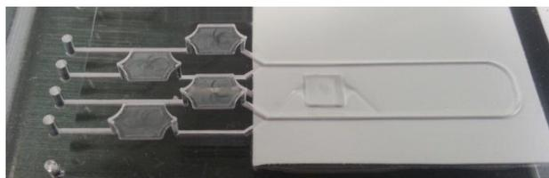
Fig. 1. Microfluidic chip for solvent extraction with in-line measurement sites.
