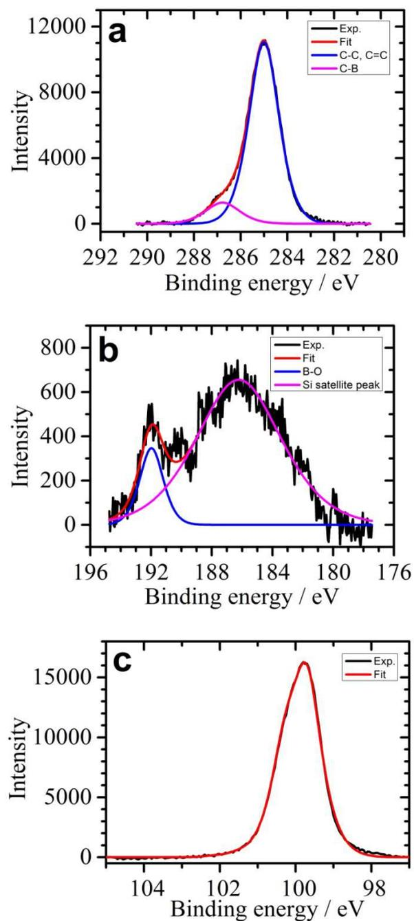
**Figure 1.** High-resolution XPS C 1s (a), B 1s (b) and Si 2p (c) spectra of **Si-EBBA**. Black lines are experimental data and red lines are the fitted curves that were generated using combinations of Gaussian-Lorentzian functions, each corresponding to a different contribution. Spectra have been recorded at 45° takeoff angle.
