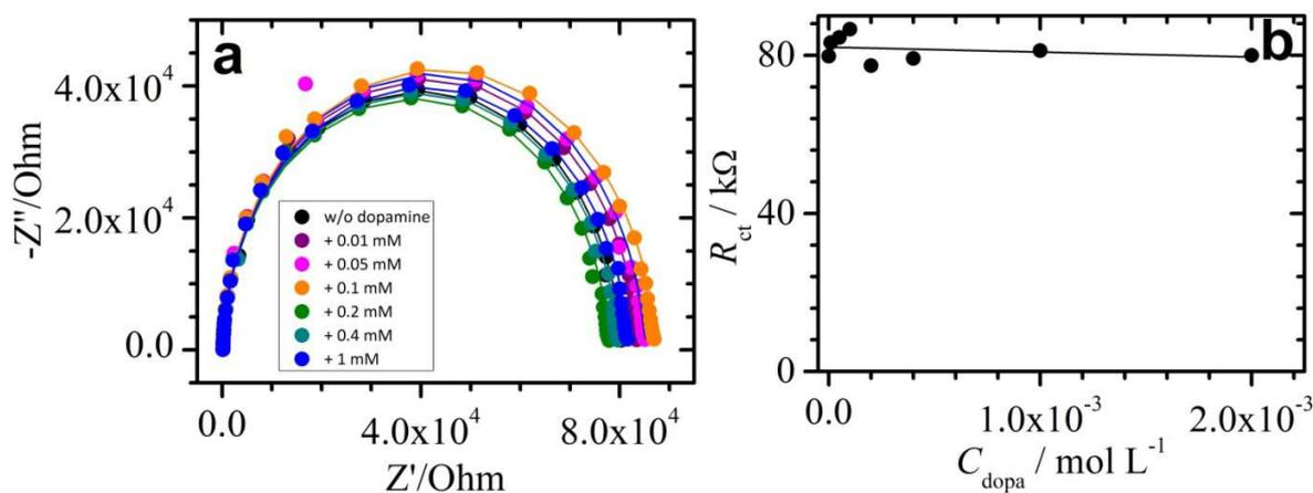
**Figure 4.** Nyquist ( $-Z''$  vs.  $Z'$ ) plots for the **Si-EB** surface at pH 7.4 + 2 mM  $\text{Fe}(\text{CN})_6^{3-}/\text{Fe}(\text{CN})_6^{4-}$  in the absence of dopamine and with increasing concentrations of dopamine (a). Applied potential: 0.15 V vs SCE. The filled dots are the experimental data and the solid lines correspond to the fitted curves assuming a Randles equivalent electrical circuit. (b) Corresponding  $R_{ct}$  – (DA concentration) plot.
