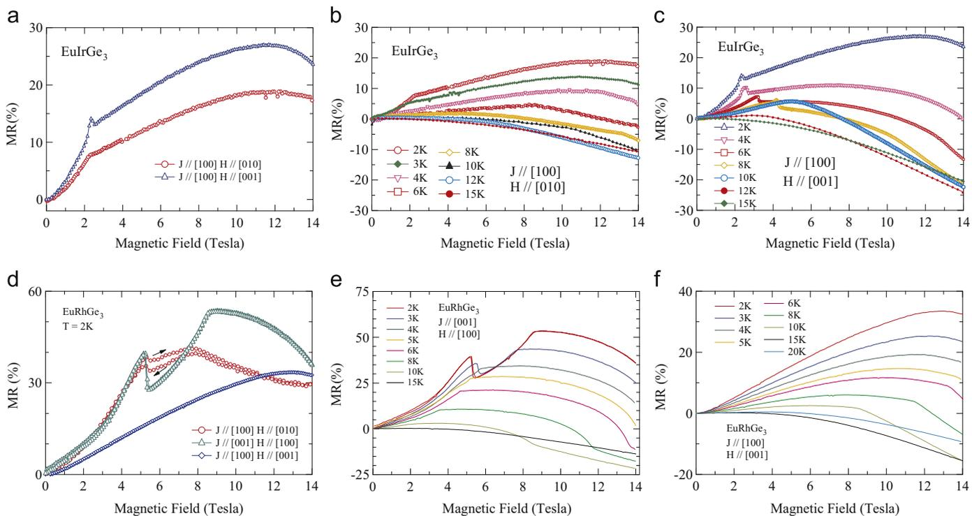
Fig. 11. The variation of magnetoresistance with field at selected temperatures in EuIrGe<sub>3</sub> (upper panels) and EuRhGe<sub>3</sub> (lower panels).
