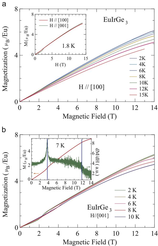
**Fig. 3.** Field dependence of magnetisation at selected temperatures in  $\text{EuIrGe}_3$  along (a) [100] and (b) [001]. Inset in (a) represents nearly isotropic magnetisation plots in  $\text{EuIrGe}_3$  and in (b) a representative derivative of magnetisation plot along [001] at 7 K (right scale) along with the  $M(H)$  data (left scale) is shown. (For interpretation of the references to color in this figure caption, the reader is referred to the web version of this paper.)
