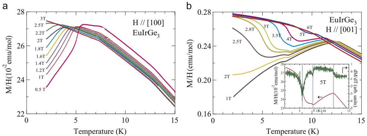
**Fig. 2.** Temperature dependence of  $M/H$  at selected fields along [100] (left panel) and [001] (right panel) for  $\text{EuIrGe}_3$ . Inset in (b) shows  $M/H(T)$  at 5 T on the left scale and its derivative on the right scale with vertical dotted line at critical points.
