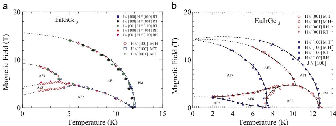
Fig. 12. H – T phase diagram of (a) EuRhGe<sub>3</sub> and (b) EuIrGe<sub>3</sub> constructed from critical points in  $M(T, H)$  and  $\rho(T, H)$  data. Solid lines are guide to the eye and dotted lines are extrapolation.
