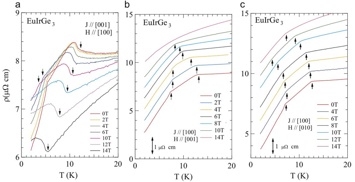
**Fig. 9.**  $\rho(T)$  of  $\text{EuIrGe}_3$  for different configurations of current and applied magnetic fields. In b and c, the traces for non-zero fields have been moved in vertical direction for clarity. Arrows indicate magnetic phase transitions. (For interpretation of the references to color in this figure caption, the reader is referred to the web version of this paper.)
