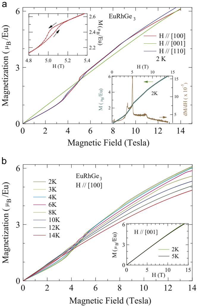
Fig. 6. (a) Isothermal magnetisation  $M(H)$  at 2 K of  $\text{EuRhGe}_3$  along the principal crystallographic directions. Bottom inset shows  $M(H)$  at 2 K on left scale and its derivative on right scale revealing field induced spin reorientations. (b) Temperature evolution of  $M(H)$  of  $\text{EuRhGe}_3$  along [100] in main panel and along [001] in the inset. (For interpretation of the references to color in this figure caption, the reader is referred to the web version of this paper.)
