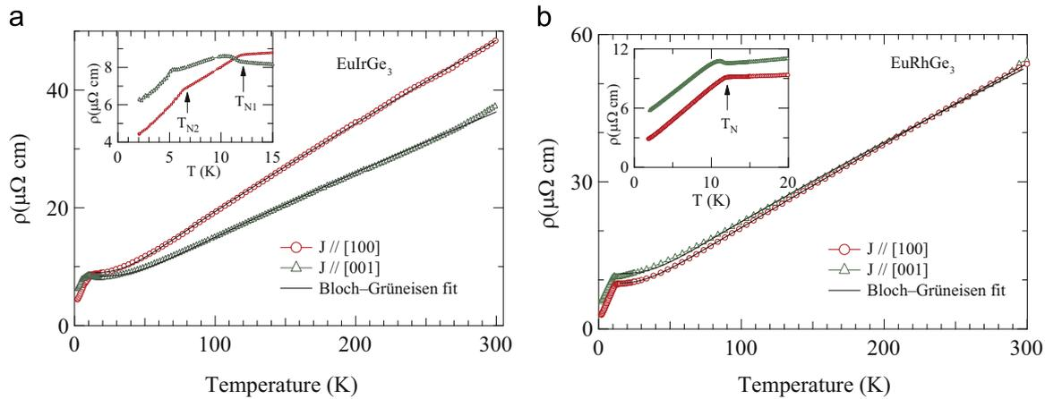
**Fig. 8.** Variation of electrical resistivity ( $\rho(T)$ ) for current density  $J_{\parallel}$  [100] and [001] for (a)  $\text{EuIrGe}_3$  and (b)  $\text{EuRhGe}_3$ . Insets show low temperature data on an expanded scale where the magnetic transitions are marked by arrows.
