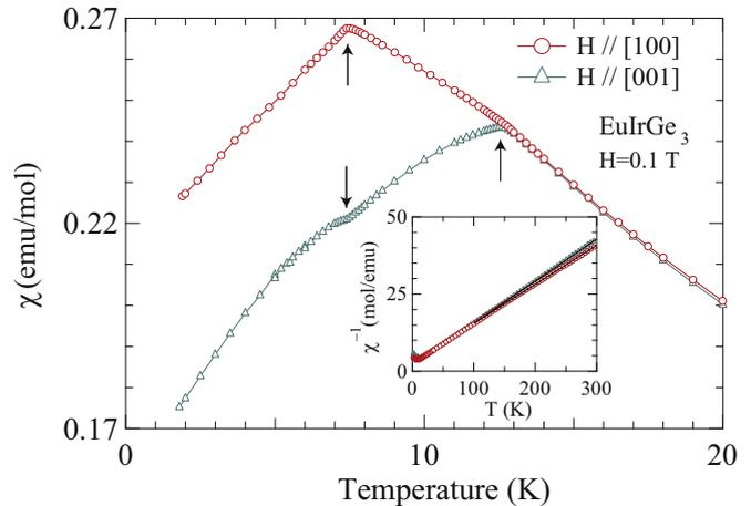
Fig. 1. Magnetic susceptibility and inverse magnetic susceptibility (in inset) of EuIrGe<sub>3</sub> at field 0.1 T along [100] and [001].
