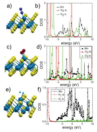
Fig. 7 Equilibrium geometry of different adsorbed molecules on a defective  $MoS_2$  monolayer (a)  $N_2$ , (c)  $O_2$  and (e)  $H_2$ . In (b), (d) and (f) the DOS of the Mo atom (black square) bonded to each molecule (green triangles) are shown together with the DOS of the isolated molecule for  $N_2$ ,  $O_2$  and  $H_2$ , respectively. The Fermi energy is fixed at 0 eV.
