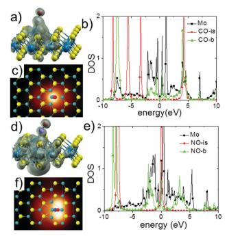
Fig. 5 Real-space electronic density integrated between -0.5 and 0.5 eV with the equilibrium geometry of different adsorbed molecules on a defective  $MoS_2$  monolayer like (a) CO and (d) NO. In (b) and (e) the DOS of the Mo atom (black square) bonded to each molecule (green triangles) are shown together with the DOS of the isolated molecule for CO and NO, respectively. The Fermi energy is fixed at 0 eV. The STM image simulated at V = -1.0 V is presented in (c) and (f) for CO and NO.
