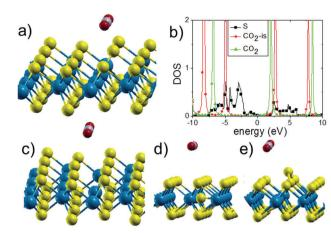
Fig. 3 Equilibrium geometry of a CO<sub>2</sub> molecule physisorbed on a MoS<sub>2</sub> monolayer with (a) S vacancy, (c) Mo vacancy, (d) and (e) one and two S substitutional atoms occupying a Mo vacancy; (b) DOS of a S atom far away from the vacancy (black squares), the  $CO_2$  placed over the S vacancy (green triangles) and the isolated molecule (red circles). The Fermi energy is fixed at 0 eV
