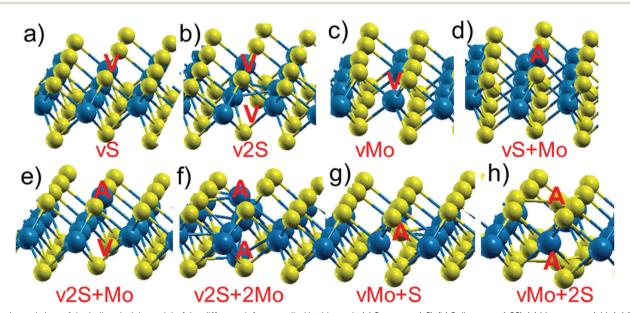
Fig. 2 Lateral view of the ball and stick model of the different defects studied in this work: (a) S vacancy (vS), (b) S divacancy (v2S), (c) Mo vacancy (vMo), (d) a Mo atom occupying the S vacancy (vS + Mo), (e) and (f) one (v2S + Mo) and two Mo (v2S + Mo2) atoms occupying the S divacancy, respectively, and (g) and (h) the same for S atoms in the Mo vacancy (vMo + S and vMo + S2 respectively). The vacancy sites and antisites are indicated with V and A labels respectively.
