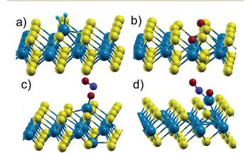
Fig. 9 Atomic representation of the dissociative configurations of different molecules on a defective MoS<sub>2</sub> monolayer: (a) H<sub>2</sub> dissociated on the substitutional Mo atom occupying a S vacancy, (b) O2 molecule dissociated in a Mo vacancy, (c) NO<sub>2</sub> over two Mo atoms occupying the S-divacancy and (d) NO<sub>2</sub> over a Mo substitutional atom on a S vacancy
