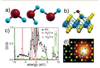
Fig. 6 (a) The three orientations of the water molecule studied in this work are presented; (b) equilibrium geometry of a water molecule adsorbed on a defect formed by two substitutional Mo atoms on a S divacancy on a  $MoS_2$  monolayer. (c) DOS of the Mo atom (black square) bonded to the water molecule (green triangles) and DOS of the isolated molecule (red circles). The Fermi energy is fixed at 0 eV. The STM image simulated at V = -1.0 V is presented in (d).
