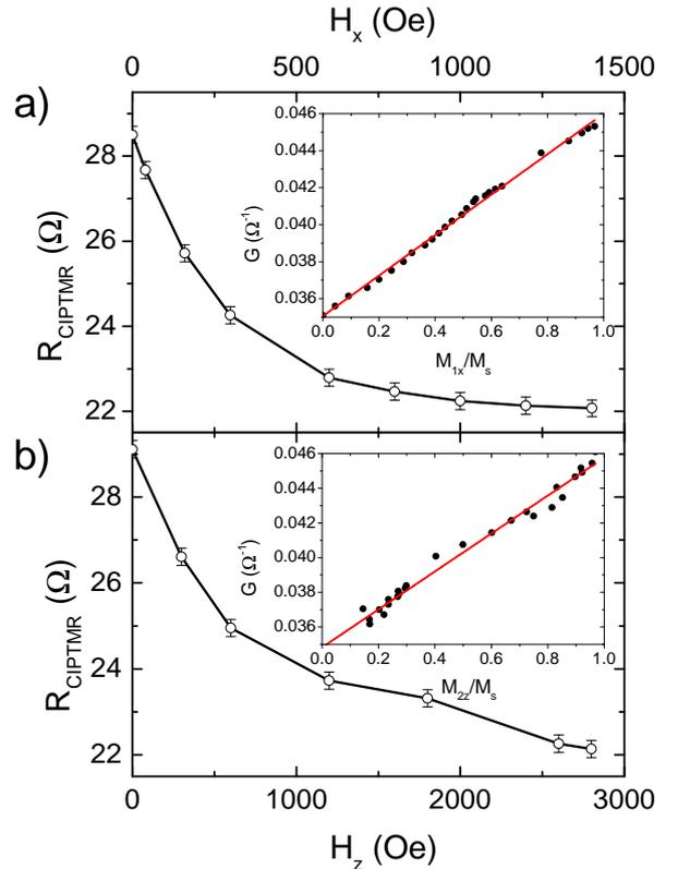
FIG. 4:  $R_{\text{CIPTMR}}$  versus field. a) Field applied in-plane (x-direction); (b) Field applied out-of-plane (z-direction). Inset: Conductance (inverse of  $R_{\text{CIPTMR}}$ ) versus the reduced component of the rotating magnetization along the applied field direction. The red line represents a linear fit of the experimental variation.
