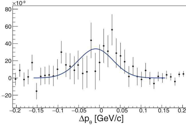
FIG. 10. Count rate differences for antiparallel vs parallel beam and target polarization for the  $\text{ND}_3$  target, vs  $\Delta p_\theta$ . The distribution is fit with a free scale parameter for both D and H. The lowest  $\chi^2$  results from a fit with no contribution from free protons.
