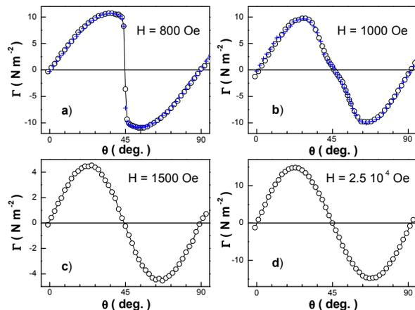
FIG. 6: Torque for  $T = 215$  K. Circles are for increasing  $\theta$ ; crosses, for decreasing ones. Note the difference in the torque scale. Conventions for  $\theta$  and  $\Gamma$  are displayed in Fig. 5.
