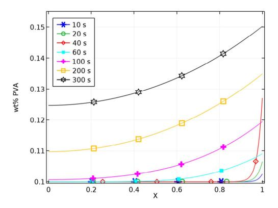
Concentration profiles simulated by the model - Ti = 20 °C, Tf = 60 °C, RH = 50%, Tramp = 35 °C/min, Casting thickness = 1 mm Fig. 6  $135 \times 101 \text{mm} \ (150 \times 150 \ \text{DPI})$
