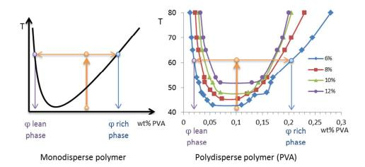
Phase diagram and coexistence curves pour PVA versus monodisperse polymer Fig. 3  $163x83\text{mm (}150\ x\ 150\ \text{DPI)}$
