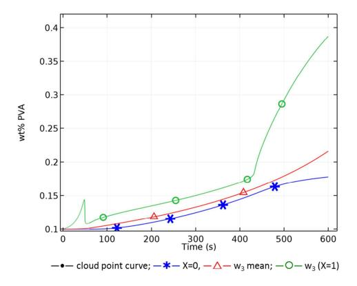
Weight fraction of PVA versus time - Ti = 20 °C, Tf = 60 °C, RH = 50%, Tramp = 35 °C/min, Casting thickness = 1 mm Fig. 7 143x119mm~(150~x~150~DPI)
