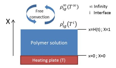
Schematic of LCST-TIPS process Fig. 2  $95x70mm (150 \times 150 DPI)$
