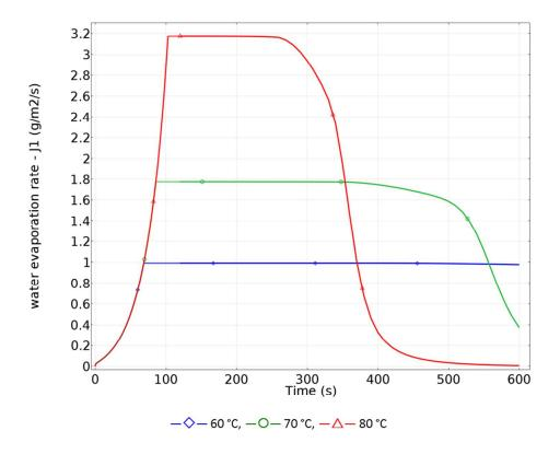
Water evaporation flux - Ti = 20 °C, Tf = 60 °C, 70 °C and 80 °C, RH = 50%, Tramp = 35 °C/min, casting thickness = 1 mm Fig. 10 174x140mm~(150~x~150~DPI)
