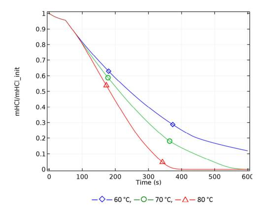
Loss of HCl during membrane formation – ratio between HCl mass at time t to initial HCl mass - Ti = 20 °C, Tf = 60 °C, 70 °C and 80 °C, RH = 50%, Tramp = 35 °C/min, casting thickness = 1 mm Fig. 11 139x117mm~(150~x~150~DPI)
