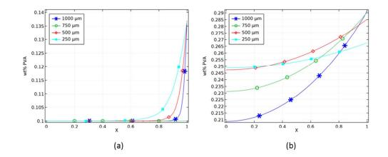
PVA concentration profiles for increasing initial solution thickness; (a) just before the composition path enters the diphasic region; (b) just before the composition path leaves the diphasic region - Ti = 25 °C, Tf = 80 °C, Tf = 80
