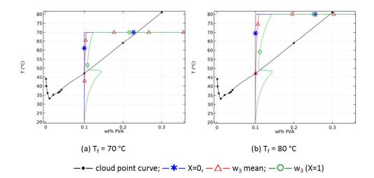
Composition path simulated by the model - Ti = 20 °C, Tf = 70 and 80 °C, RH = 50%, Tramp = 35 °C/min, Casting thickness = 1 mm Fig. 8  $167x88mm~(150\times150~DPI)$
