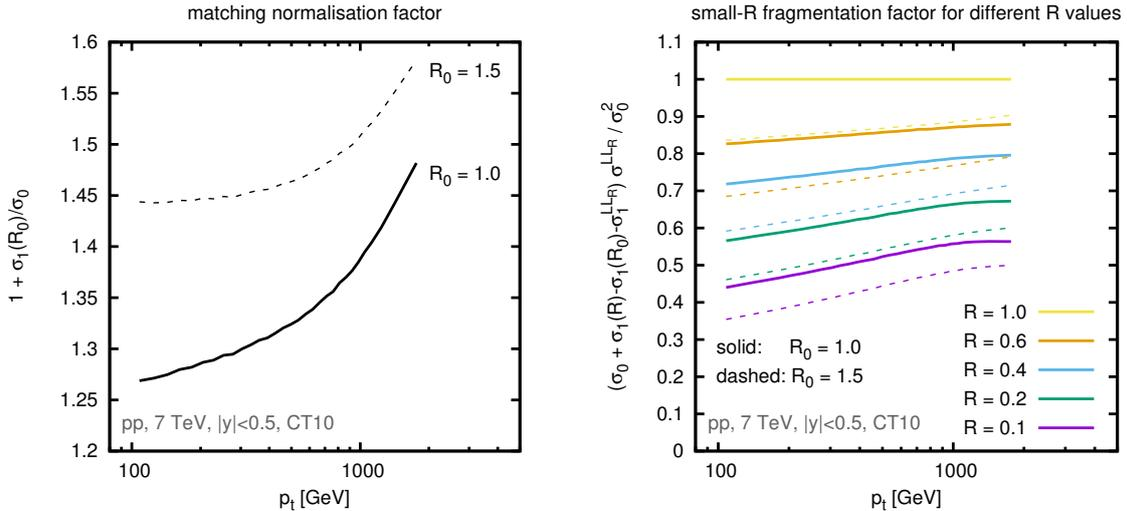
**Figure 3.** Left: size of the matching normalisation factor (left-hand factor of Eq. (3.4), normalised to LO), shown v.  $p_t$  for various  $R$  values and two  $R_0$  choices. Right: size of the matched small- $R$  fragmentation factor (right-hand factor of Eq. (3.4); similar results are observed for the right-hand factor of Eq. (3.5)). The results are shown for the scale choice  $\mu_R = \mu_F = p_{t,\max}$ , where  $p_{t,\max}$  is the transverse momentum of the hardest jet in the event.
