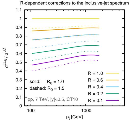
**Figure 1.** Impact of  $R$ -dependent terms in the inclusive-jet spectrum, illustrated using the small- $R$  resummation factor obtained from the ratio of  $\sigma^{LLR}$  in Eq. (2.1) to the leading order inclusive jet spectrum  $\sigma^{LO}$ . It is shown as a function of the jet  $p_t$  for different jet radius values. For each  $R$  value, the plot illustrates the impact of two choices of  $R_0$ :  $R_0 = 1$  (our default) as solid lines and  $R_0 = 1.5$  as dashed lines.
