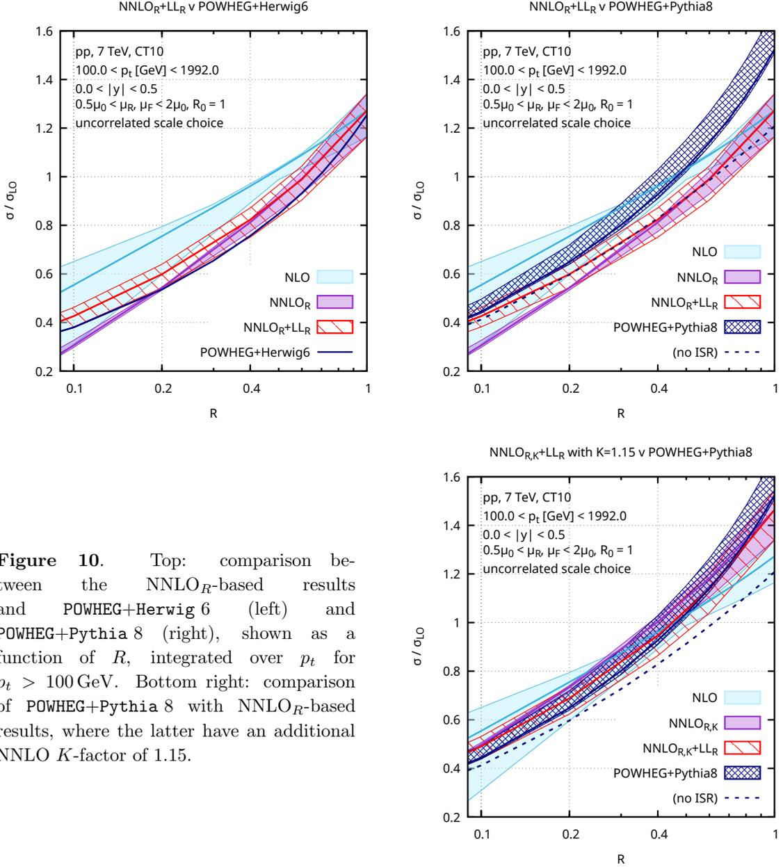
**Figure 10.** Top: comparison between the NNLO<sub>R</sub>-based results and POWHEG+Herwig 6 (left) and POWHEG+Pythia 8 (right), shown as a function of  $R$ , integrated over  $p_t$  for  $p_t > 100$  GeV. Bottom right: comparison of POWHEG+Pythia 8 with NNLO<sub>R</sub>-based results, where the latter have an additional NNLO  $K$ -factor of 1.15.
