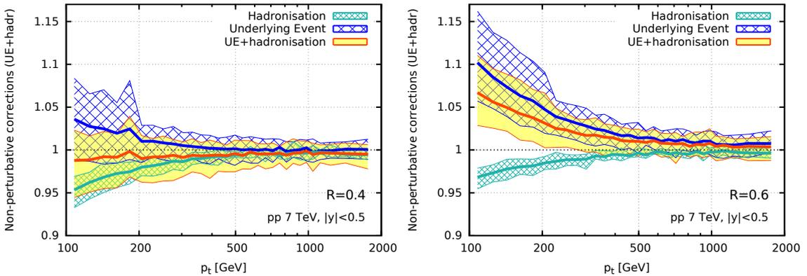
**Figure 16.** Non-perturbative corrections to the inclusive jet spectrum for the  $p_t$  range, rapidity and centre-of-mass energy corresponding to the ATLAS data [26] for  $R = 0.4$  (left) and  $R = 0.6$  (right).
