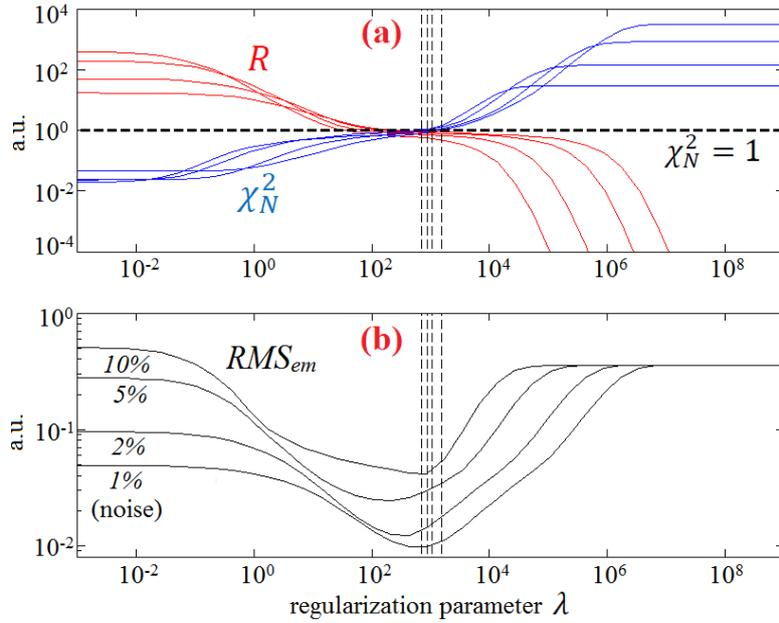
Figure 4.  $\lambda$  optimization with the Gaussian phantom and different noise levels with (a) residual  $\chi_N^2$ , regularization term  $R$  and (b) reconstruction error  $RMS_{em}$  versus  $\lambda$ . Vertical dashed lines correspond to the solution of Eq. (2.5).
