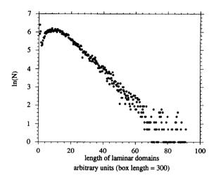
Fig. 13. Typical behavior of the distribution of laminar lengths, computed from a sample of 3000 consecutive states (distant from each other by one unit of time) of the 1D system. Here  $\mu = 1$ ,  $\alpha = 1$ ,  $\beta = -1.6$ ,  $\gamma = 0.5$ ,  $\delta = 0.3$ ,  $\xi = 1$ ,  $\eta = 1$  and  $\kappa = 1$ .
