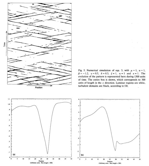
Fig. 6. Amplitude (a) and phase (b) of one of the traveling dips in fig. 5. The value of |A| at the center of the dip and the amplitude of the "phase jump" change as the dips propagates.
