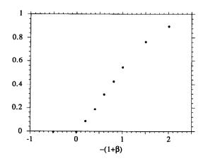
Fig. 11. Behavior of the turbulent fraction  $F_t$  as a function of the order parameter  $-(1+\beta) \alpha |D|$ . Measurements have been made from samples consisting of 3000 consecutive states (distant from each other by one unit of time) of the 1D system, and for various values of  $\beta$ . Other parameters were kept constant (see text).
