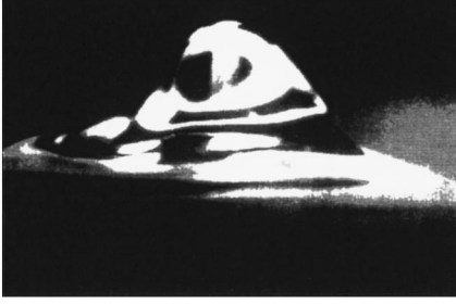
FIG. 2. Picture of a rotating bump for U > U_c . The jet diameter is equal to 1 mm, the height and width of the bump are of the same order, about 3 mm.
