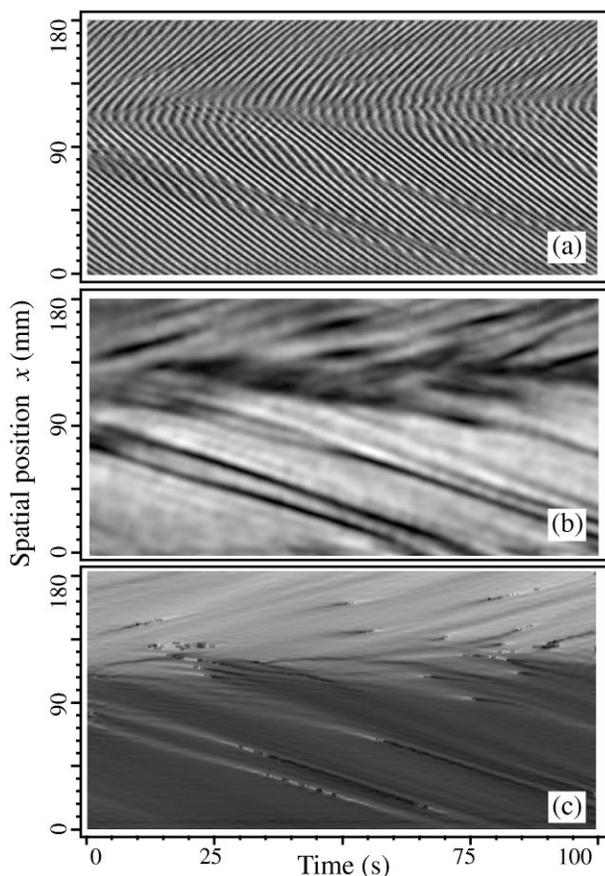
FIG. 2. Spatiotemporal evolution of the wave pattern at  $h = 1.2$  mm and  $\Delta T = 5.1$  K (yielding a Marangoni number  $\text{Ma} = 950$ ). Only a central portion of length 18.5 cm is shown during 100 s. (a) Original data; (b) evolution of the modulus  $|A|$  (black:  $|A| = 0$ ; white:  $|A| = 1$ ); and (c) phase gradient  $k$  (dark:  $k < 0$ ; bright:  $k > 0$ ).
