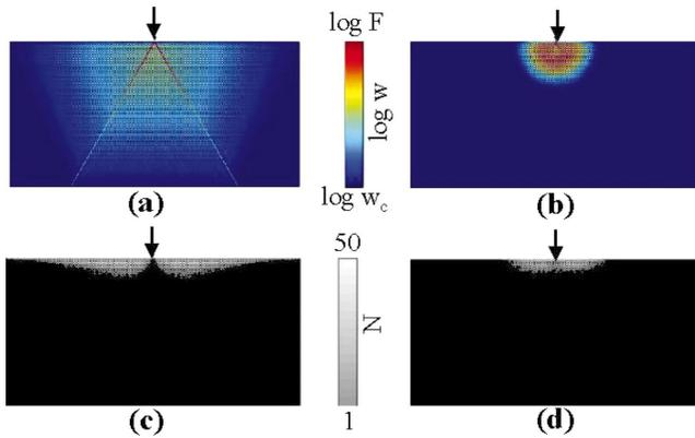
FIG. 4. (Color) Mean distribution of the overloads (top) and of the displacements (bottom) generated by the force  $F$ . Model predictions  $L$  and  $H$  have been chosen to be  $L=100$  and  $H=100$  and a numerical experiment is averaged over 50 realizations. Left:  $\Theta = 5^\circ$ . Forces propagate preferentially along two directions. Displacements are confined into two triangles on both sides of the two preferential lines. Right:  $\Theta = 30^\circ$ . The pattern disappears.
