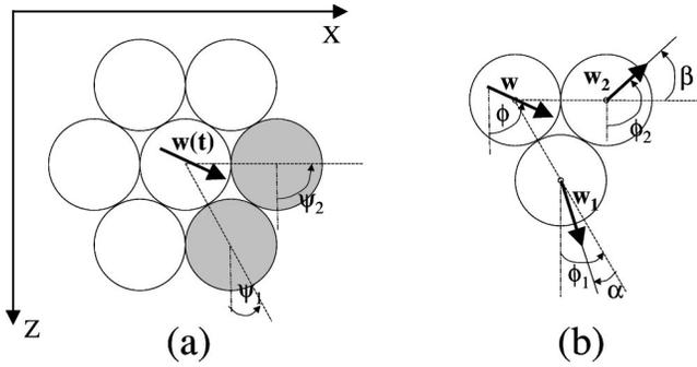
FIG. 3. Propagation rule of the overload from a given bead to two of its neighbors. (a) The orientation  $\phi$  of the load  $\mathbf{w}$  determines the two neighbors  $P_1$  and  $P_2$  which will support this charge. (b) The orientations  $\phi_1$  and  $\phi_2$  of the two *children* charges resulting from the transmission coincide with the two contact orientations  $\psi_1$  and  $\psi_2$  at which two random numbers  $\alpha$  and  $\beta$  have been added, respectively.
