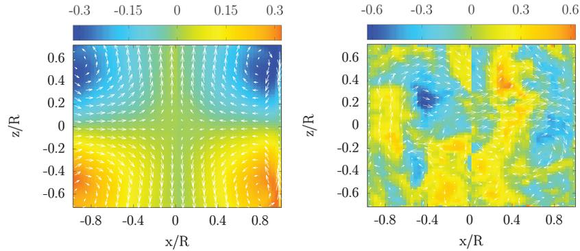
FIG. 1. Left, time-averaged velocity field  $\bar{\mathbf{v}}$ , measured in a meridional plane using S-PIV, at  $\text{Re} = 10^6$  and  $\theta = (f_1 - f_2)/(f_1 + f_2) = 0$ .  $x = r \cos \varphi_0$ ,  $\varphi_0 = [0, \pi]$ . Right, corresponding instantaneous fluctuating component of the velocity field  $\mathbf{v}' = \mathbf{v} - \bar{\mathbf{v}}$ . The color maps the azimuthal velocity  $v_\varphi$  (normalized by  $R(f_1 + f_2)/2$ ) whereas the arrows map the  $(v_x, v_z)$  velocities.
