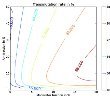
Fig. 3. Transmutation rate versus fraction of moderator.
