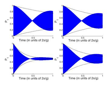
FIG. 7. (Color online) Probability of finding the reduced flux qubit density matrix in the excited state  $|1\rangle$  as a function of time (in units of  $2\pi/g$ ).  $T_{\nu} = 15 \ \mu$ s while  $T_1$  is 20, 10, 5, and 2  $\mu$ s (from top left, decreasing clockwise). Black crosses show the envelope of the fast oscillations in the absence of coupling g = 0.
