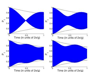
FIG. 6. (Color online) Probability of finding the reduced flux qubit density matrix in the excited state  $|1\rangle$  as a function of time (in units of  $2\pi/g$ ). Decoherence is modeled through  $T_1 = 20 \ \mu s$ ,  $T_{\nu} = 15 \ \mu s$ . Black crosses show the envelope of the fast oscillations in the absence of coupling g = 0. From top left, and increasing clockwise, values of the detuning are  $\Omega + \delta = 0, g/2, g$ , and 2g.
