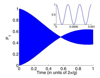
FIG. 4. (Color online) Probability of finding the flux qubit in the excited state as a function of time (in units of  $2\pi/g$ ), for a spin initial state  $|1\rangle$ . Time evolution is computed in the laboratory frame. The plot is at resonance condition; decoherence is  $T_1 = 20 \ \mu s$ ,  $T_{\nu} = 15 \ \mu s$ . (Inset) Zoom on the fast Rabi oscillations for very short times.
