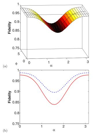
FIG. 9. (Color online) Fidelity of the NV center reduced density matrix after the protocol with the initial flux qubit state (a) as a function of  $\alpha$  and  $\phi$  and (b) as a function of  $\alpha$  only. (a) Shows that the fidelity of the protocol is actually  $\phi$  independent. Values of decoherence for the two plots in (b) are the same as in Table I.
