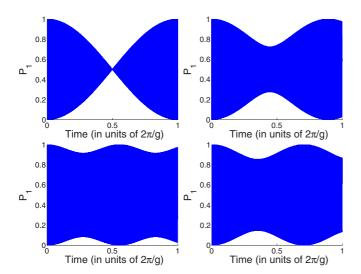
FIG. 5. (Color online) Probability of finding the reduced flux qubit density matrix in the excited state  $|1\rangle$  as a function of time (in units of  $2\pi/g$ ). Decoherence here is not taken into account. From top left and increasing clockwise, values of the detuning are  $\Omega + \delta = 0, g/2, g$ , and 2g.
