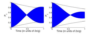
FIG. 8. (Color online) Probability of finding the reduced flux qubit density matrix in the excited state  $|1\rangle$  as a function of time (in units of  $2\pi/g$ ). Decoherence is modeled through  $T_1 = 20 \ \mu s$ ,  $T_{\nu} = 15 \ \mu s$ . Black crosses show the envelope of the fast oscillations in the absence of coupling g = 0. (Left) Spin initial state is  $|0\rangle$ . (Right) Spin initial state is  $|1\rangle$ .
