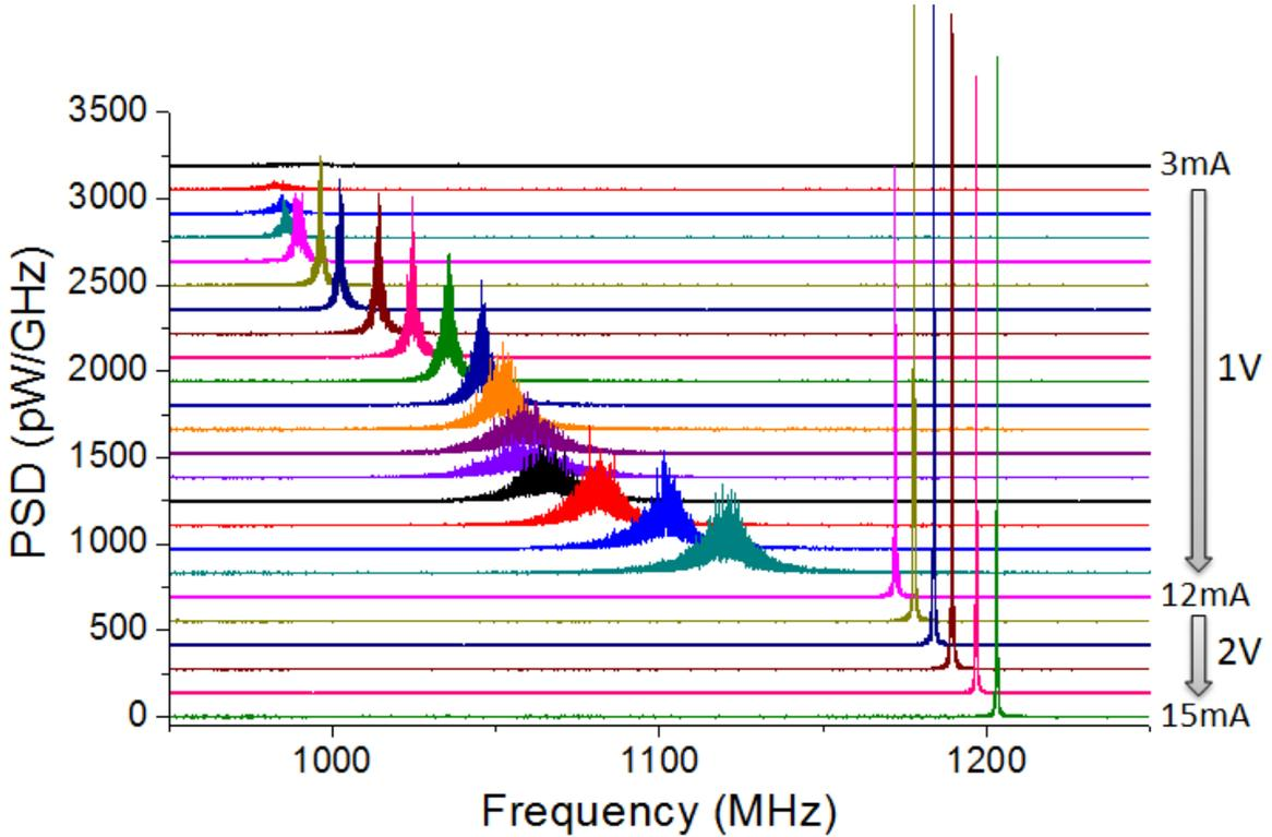
Fig. 2. Power spectrum map measured for our spin valve STNO for increasing  $I_{dc}$  in the case of a transition from a single vortex configuration to a two-vortices configuration with opposite polarities. The measurement is made under in-plane external field  $B = 34mT$ . For this field value, the transition between the two configurations happens at  $I_{dc} = 11.5mA$ . Peaks observed at harmonics of the fundamental frequency are not presented on this graph.
