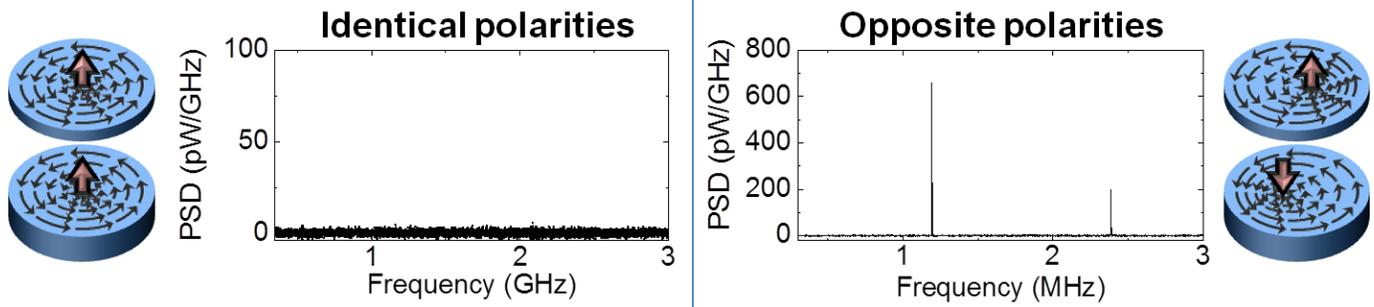
Fig. 4. Spin-valve voltage spectrum measured in the two-vortices configuration in the case of (a) identical and (b) opposite polarities, both measured at  $I_{dc} = 15\text{mA}$  and zero magnetic field.
