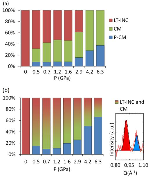
FIG. 6. (Color online) Pressure-induced magnetic phase separation in  $\text{YMn}_2\text{O}_5$  at low temperature ( $\leq 5$  K). The relative amounts of the LT-INC, CM, and PCM phases are deduced (a) from the refined diffraction patterns and (b) from the intensity of selected peaks, plotted on the right.
