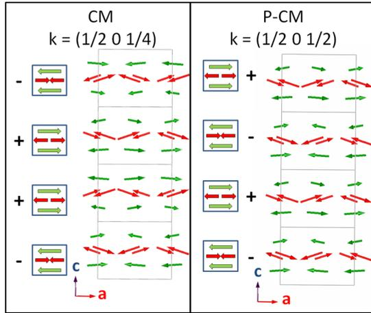
FIG. 4. (Color online) Schematic drawing of the Mn moment orientations in the CM and PCM phases in the  $ac$  plane; green and red arrows correspond to  $\text{Mn}^{4+}$  and  $\text{Mn}^{3+}$  moments, respectively; a simplified drawing of the stacking sequence of magnetic moments along the  $c$  axis is also drawn.
