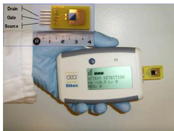
Fig. 2. Picture of the device. Insert shows the field effect transistor wire bonded on a card with the three connectors.
