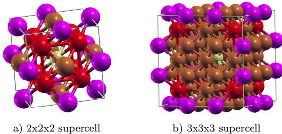
FIG. 1: (Color online) The  $2 \times 2 \times 2$  and  $3 \times 3 \times 3$  supercells with the vacancy in the corner. Different colors indicate the atom nearest to the vacancy (red), the second nearest (purple), and the furthest (the central atom, yellow).
