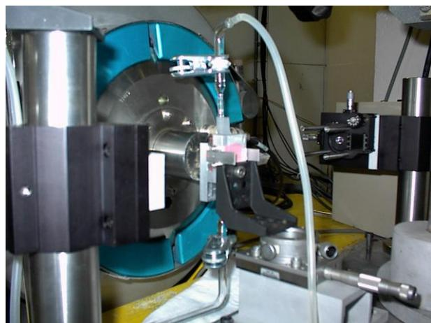
**Figure 1.** Setup for pulse radiolysis at GANIL (Experiment n°P492 on 19<sup>th</sup> of June 1999). Center of the picture: a vertical optical cell made of fused silica is irradiated with horizontal beam downstream the output “nose” of the machine made of a thin titanium foil.
