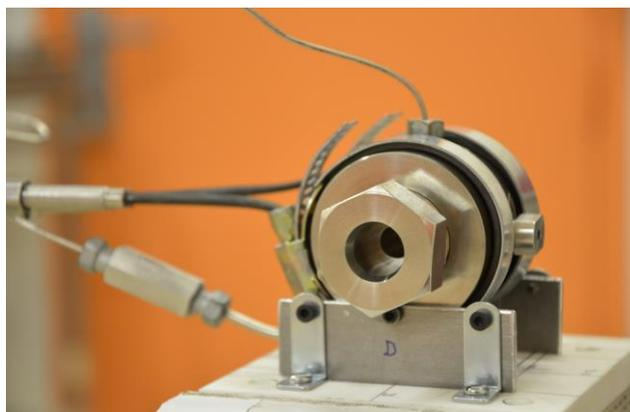
**Figure 5.** High temperature optical flow cell dedicated to Heavy ion irradiations. Imagine the ion beam come from the right side; ions enter in the hole of 3mm diameter to access the internal interaction chamber of 1.5mm of diameter. The main body is made of Inconel 718 in a 51 mm long and 51 mm diameter cylinder. Heaters (with their own thermocouples) and tubes are also going to the left. The picture does not include the main thermocouple and thermal protection made of silica wool.
