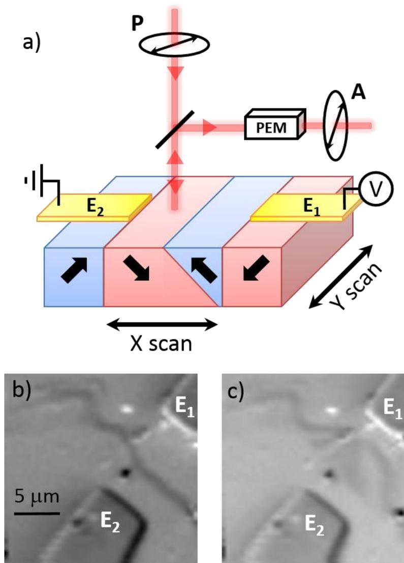
**Figure 2:**a) Schematics of the optical measurement where a focused laser spot is scanned on the sample and two quantities are recorded including the change of light polarization and the current extracted through the electrodes. The latter allows to map the photocurrent generation while the former gives the ferroelectric domain configuration as shown on the two images (b and c) where the dark line corresponds to the domain wall.
