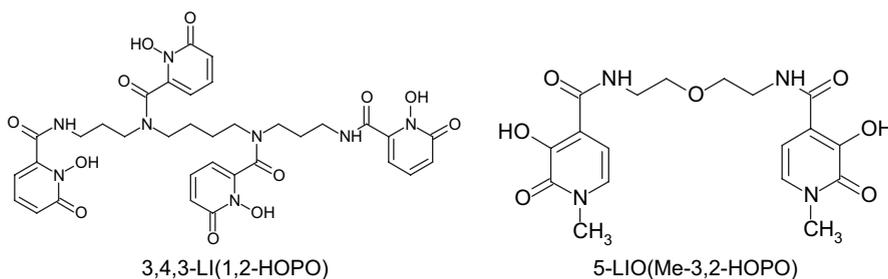
Fig. 1. Examples of two efficient hydroxypyridonate compounds.
