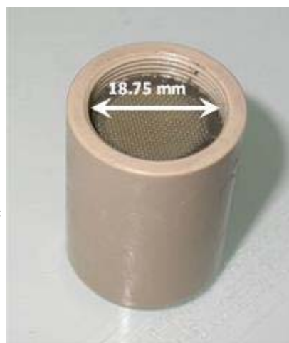
Figure 65 Schematic representation of the through-diffusion cell used with radiotracers (left). The micro-cell used for the in-diffusion experiment (right) (Frasca et al., 2012).
